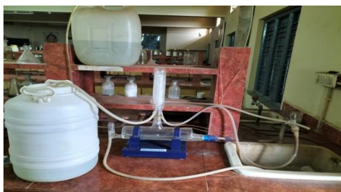
Distilled water plant
